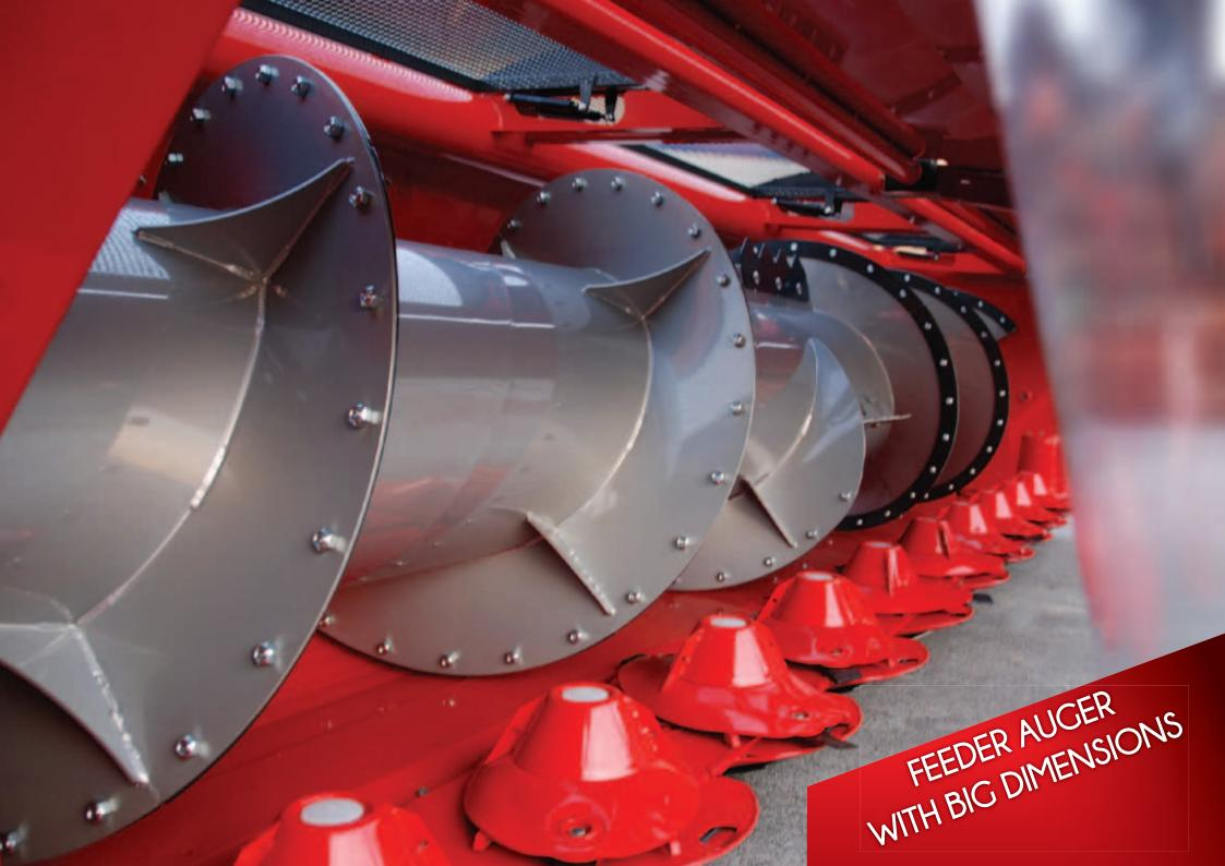
The SPARTAN can be attached to any self-propelled forage harvester and its floating feeder auger with a large diameter allows regular product flow in different products, even under the most difficult conditions. Another advantage is the easy exchange of the highly resistant wearing parts.
